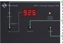
926 Factor Button Factor conversion to Salt concentration. (9265 Switch Selects sample volume 100µL/20µL).
