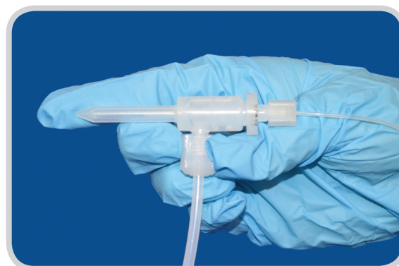
Clearing a Blockage by Backflushing a C-Flow. No Need for Tools or Wires. Simply Place a Gloved Finger Over the Tip While Ar Nebulizer Gas is Flowing.
