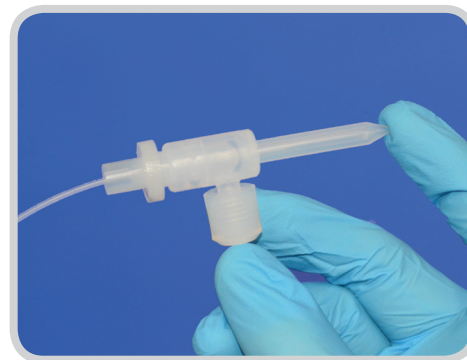
Backflushing a C-Flow Nebulizer
