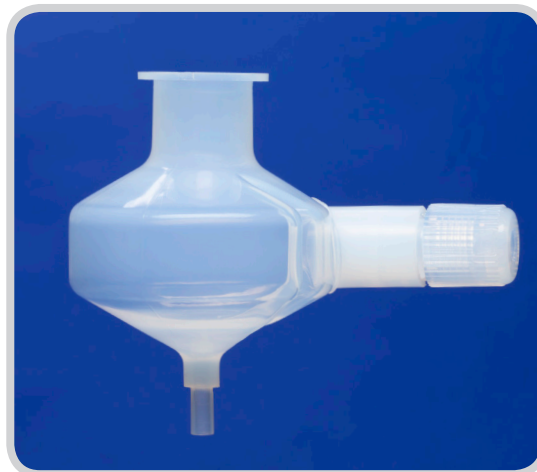
Side view of the PFA CSC (no exit port fitted) showing deep spoiler molded into sidewall
