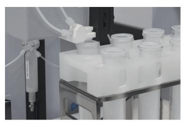
**NovaWAVE** Teflon® vessels, HF acid, and HNO<sub>3</sub> acid being added prior to microwave digestion, will work with any microwave Teflon® vessels.
