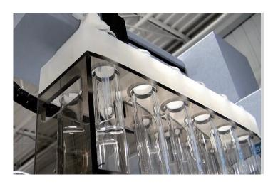
**NovaWAVE** calibrated quartz tubes being normalized and filled to volume automatically.
