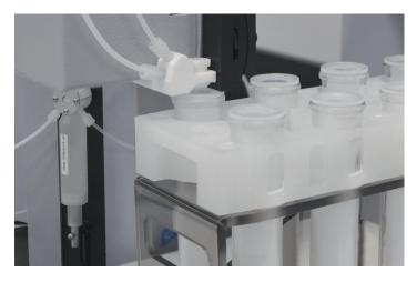
Digestion acids can be added in multiple steps to prevent vigorous reactions.
