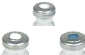
Crimp too tight
