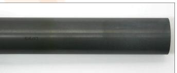
By contrast, the ceramic material does not devitrify and is not affected by salt deposits. The ceramic D-Torch in the photo was run for the same period and with the same samples as the quartz torch but shows no degradation at all.
