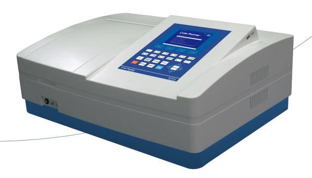
The SP-800-UV is a UV-Visible double-beam spectrophotometer with a variable spectral bandwidth. The spectrophotometer has an integrated user interface for local control and ease of navigation. The highly stable optics and two detectors measure the sample and reference simultaneously, optimizing measurement accuracy.
